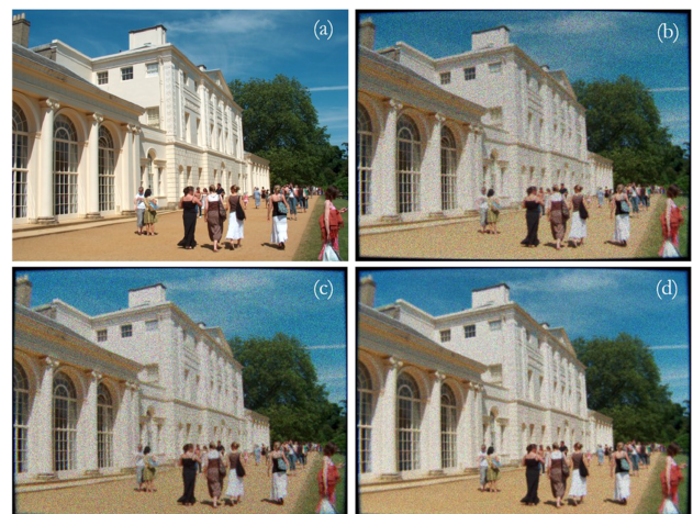
Fig. 4. (a) Input image is shown alongside simulated images from the (b) top, (c) bottom, and (d) back-side sensor.
